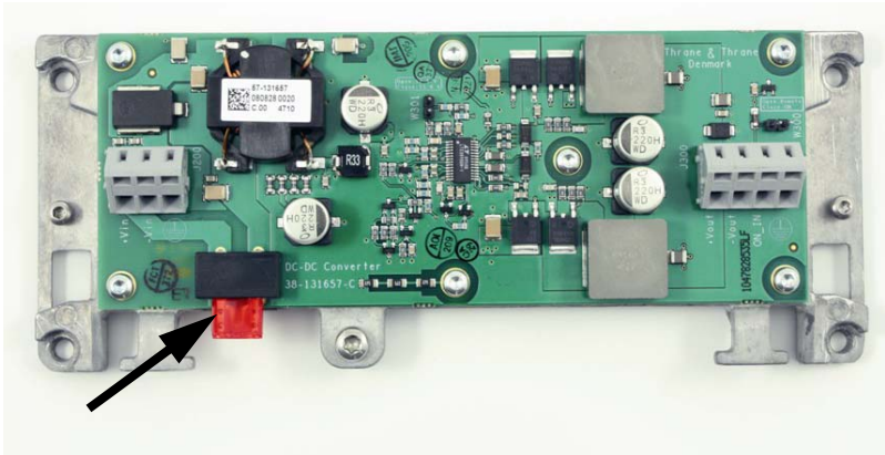
Figure 4: Replacing the fuse in the Power Converter
