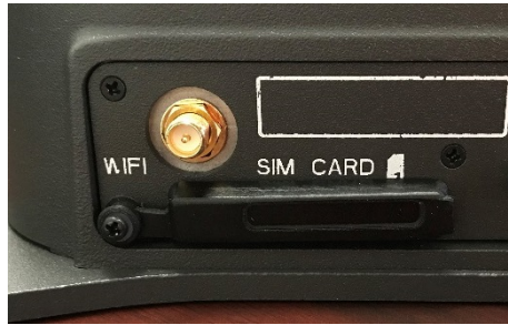
Figure 3-5 Secure the SIM Card Cover
