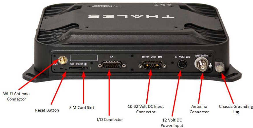
Figure 2-7 Below Deck Unit (BDU) Back Panel Detail
