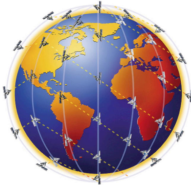
Figure 1-1 Earth showing Iridium satellites in six defined orbital planes.
